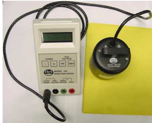
Figure 4: Surface resistivity measurement setup.
